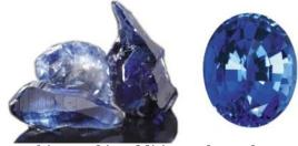
In 1902 the French chemist Auguste Verneuil developed a process for producing synthetic sapphire crystals. In the Verneuil process, named for him, fine alumina powder is added to an oxyhydrogen flame, and this is directed downward against a mantle. The alumina in the flame is slowly deposited, creating a teardrop shaped "boule" of sapphire material. Chemical dopants can be added to create artificial versions of the ruby, and all the other natural colours of
